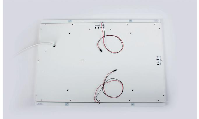
3. Place the struts on the back over the predrilled holes of the infrared heater and insert the screw threads on the profiles through the holes provided on the rail. Attach the struts to the infrared heater with the enclosed screws.
